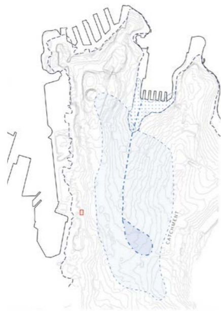
Figure 1: Tank Stream valley catchment area within Sydney CBD area. The dotted black line is the 1788 shoreline and the solid black line is the current shore line. The catchment area for the Tank Stream, the marsh at the head of the Stream, the Tank Stream itself (centre) are shown in blue. The approximate site location is at the red rectangle (Source: Yerrabingin)
